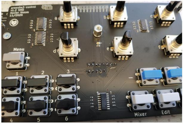
8) Step 8. Now solder the pinheaders connecting the main board and controlboard. From both sides!
