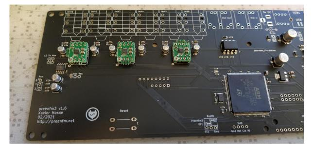
2) Step 2. Solder the jumpers, DC connector, USB connector. (in this order) TFT Vcc jumper to 5V pos.
