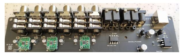
4) Step 4. Assemble the control board. Switches first, encoders last. Allign the encoders straight. Solder one leg first and then adjust them. Dont rush here.
