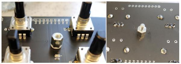
6) Step 6. Cut the precision low-profile pinheaders. Female+Male. And fit them to the main pcb. DONT SOLDER!!
