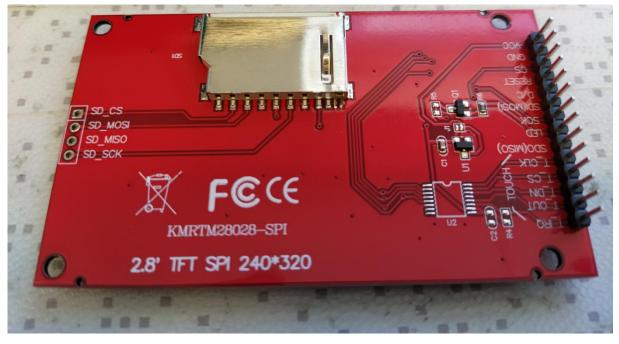
10) Step 10. Mount the TFT screen pinheaders and sockets. DONT SOLDER! Top 4 pins will be female and male together. Lower one will be only female row.
