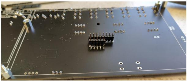
7) Step 7. Fit the control PCB on the mainboard. So that the pinheader will come through. DONT SOLDER!! Fix the board with screws and nuts to the spacers.
