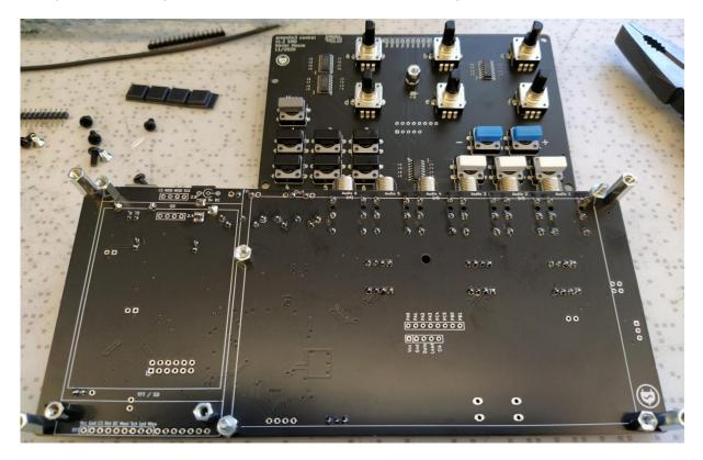
6 short Female/Male spacers for the control board mounting. (one spacer with white plastic washer) 4 long Female/Female spacers for the case.
