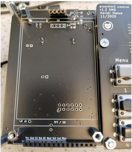
11) Step 11. Insert the TFT screen in the socet and fix with screws.
