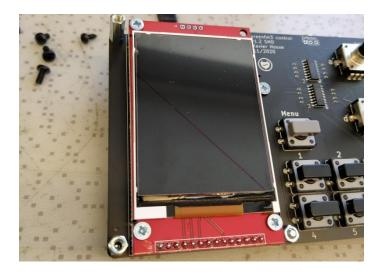
12) Step 12. Adjust the pinheaders inside the sockets. So that there is good connection. Leave gaps. Now solder all the screen pinheaders.
