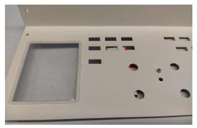
8) Step 8. Mount the Frontpanel to the PCB assembly using black 4pcs M3x6mm screws and 1pcs M3x4mm black screw. Solder the Pinheaders for the TFT screen. As many as you can reach. Make sure everything fits well. Remove the front panel from the PCB assembly and solder all the pins that you didnt reach. Also make sure you got them all. Remove the TFT screen protector film. Now put back the frontpanel.
