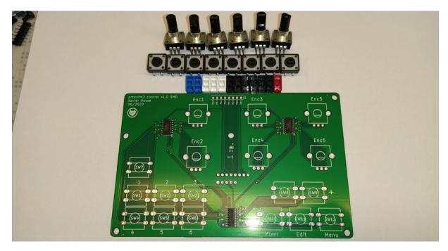
This is the result. Also install spacers 5pcs M3x6mm and 4pcs M3 nuts + M3x7mm spacer.
