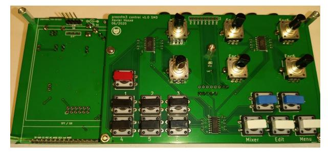
5) Step 5. Remove the short pinheader from the TFT screen and clean the holes from solder.
