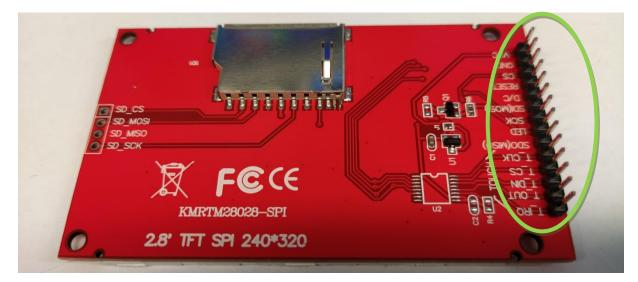
6) Step 6. Insert the TFT screen on top of the pinheaders.
