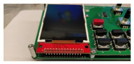
7) Step 7. Prepare the top. Remove the Plastic wrap from the Screen protector bottom, glue it with supper glue. Insert the LED Lightpipe and glue with supper glue. Let it dry.
