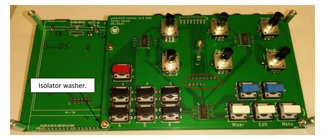
4) Step 4. Solder the pinheaders on both sides. On top of control board and on the back of the mainboard. Insert long pinheaders on the TFT position, cut 1mm off from all the pins. On the low-row cut and remove the un-needed pins. NB: Dont solder long pinheaders.
