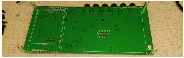
2) Step 2. Mount the switches and encoders on the control board.
