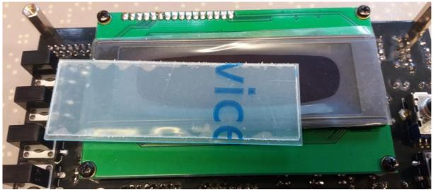
• OELD Screen pins are directly soldered to the board. So be sure its the last thing you need to do! You can even assemble the whole synt and then solder the pins as the very last thing.
