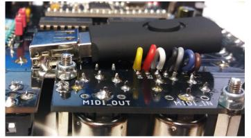
• Mount the MIDI and USB connector to the pcb and then screw to the panel. Align the connectors nicely (look from front) and then solder!
